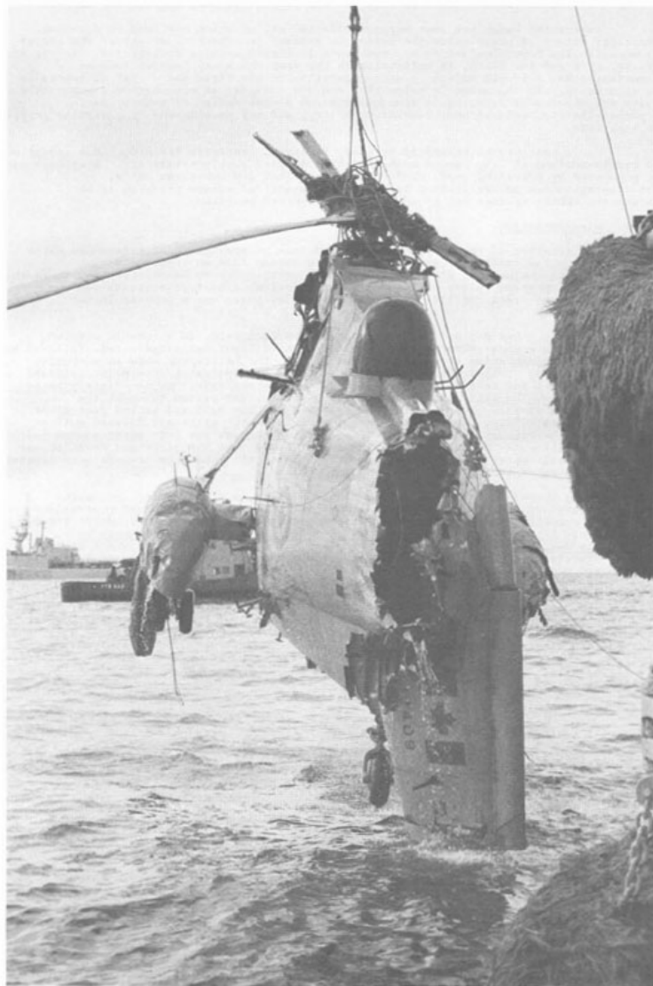
Figure 3. Typical helicopter accident in which cabin has split open on water impact.
