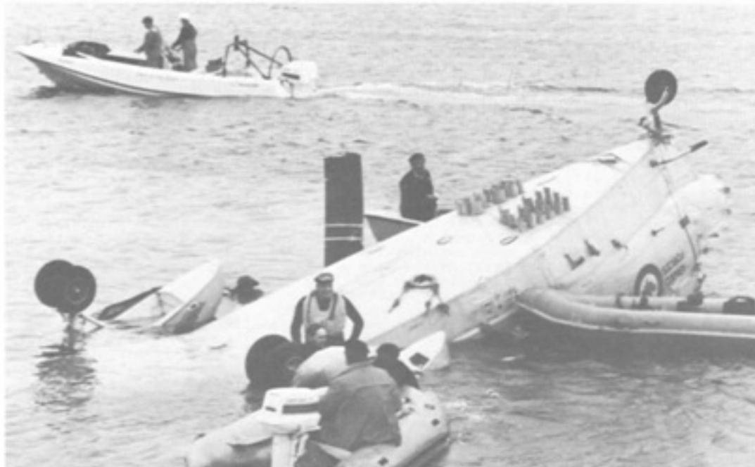
Figure 2. Typical helicopter accident where the helicopter sinks and is rapidly inverted.
