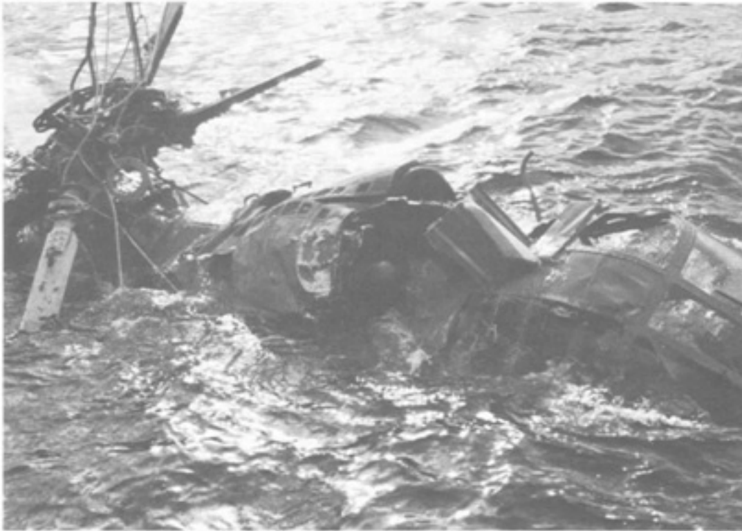
Figure 2. Typical helicopter accident where the helicopter sinks and is rapidly inverted.
